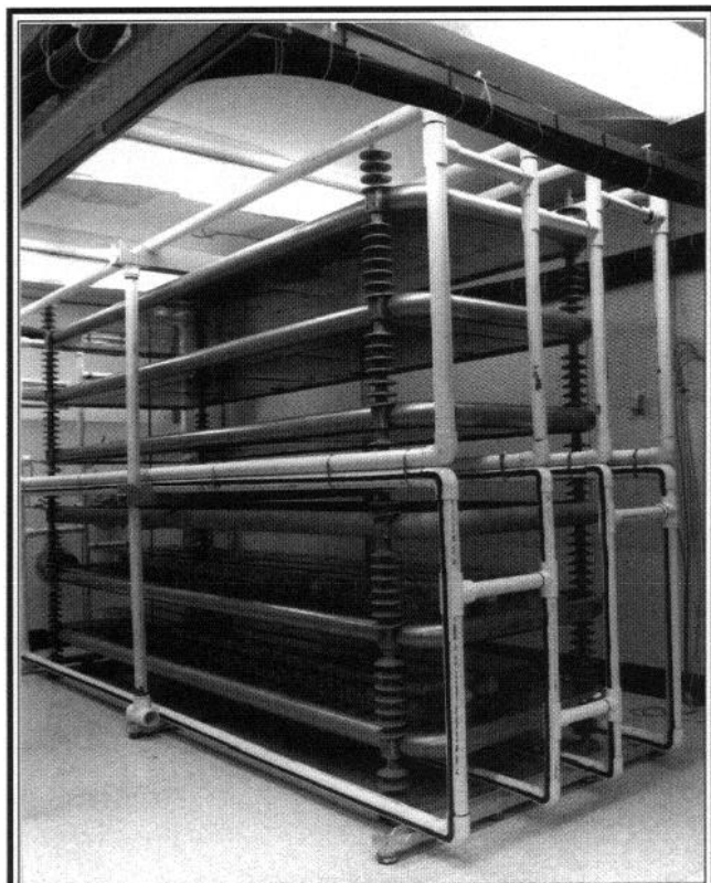
Figure 4.4. A system developed to expose laboratory animals to 60-Hz EMF. The electric field is produced by voltage on the parallel plate electrodes (metal tubing). The magnetic field is produced by current in the vertical rectangular coils (inside white plastic pipes). Photo courtesy of Battelle Pacific Northwest Labs.
