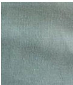
Exel is made of poly cotton interwoven with stainless steel. It is 1.5 metres wide. It shields over 99% signal strength from mobile phone mast signals (all frequencies) and also the high-band WiFi frequencies. It can be sewn easily and is opaque to light. It can be used as curtain lining, sheets or clothing
